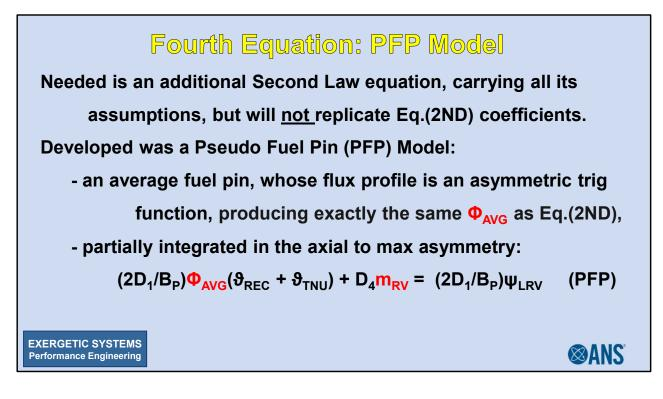
A needed fourth equation is found in another Second Law application. This is the Pseudo Fuel Pin (PFP) Model. PFP key assumptions include: it represents an average fuel pin, has an asymmetric profile, and \* is only partially integrated in the axial.
