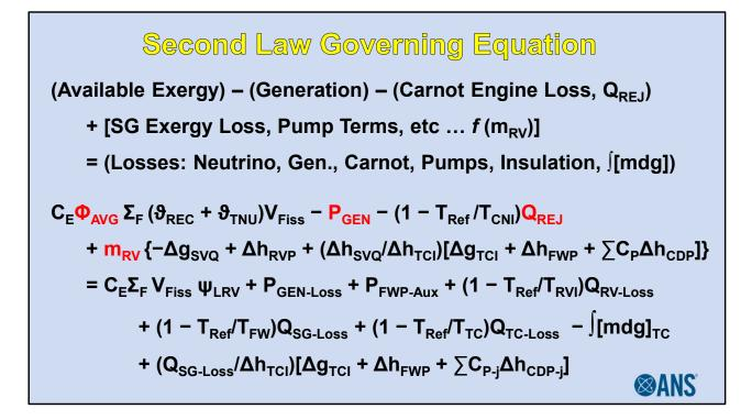
This is a NSSS Second Law balance. An  $m_{RV} \Delta g_{RVQ}$  does not appear. RV coolant flow appears only thru pump losses. \*
