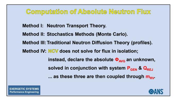
But rather, to take  $\Phi_{AVG}$  and brake shaft power to the generator, and Turbine Cycle heat rejection ... all as <u>unknowns</u> ... coupled through Reactor Vessel coolant mass flow. Thus we have <u>four unknowns</u> \* ... we need four equations.
