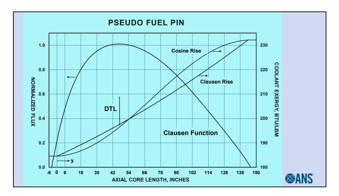
The PFP is based on the Clausen Function of Order Two. Note that an assumed cosine for the PWR will yield an essentially symmetric profile. \*
