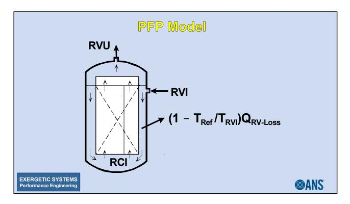
If we envision an average pin in the core, the only loss is the antineutrino. Vessel losses are associated with the outer annulus. \* By the way, the 2.6% beta & gamma coolant heating is taken into account by the recoverable release, given assumed steady state.
