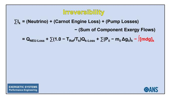
Note that classically this term describes losses associated with heat exchangers. For example, in a common feedwater heater, a decrease of m $\Delta$ g on the shell-side must be greater than an increase on the tube-side ... this produces a negative total, and thus an increase in irreversible loss. \* However, for a isolated <u>fission</u> core, all but the first term drop out.
