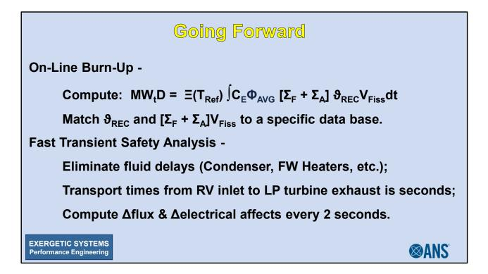
Transient analysis is viable provided the model only considers short transport times. This means the problem's boundary is reduced to the Reactor Vessel's inlet running to the LP turbine's exhaust and the generator. The electric generator should be viewed as a marvelously accurate instrument for detecting changes in neutron flux, a  $d\Phi_{AVG}/d(frequency)$ ; as based on the set of NCV equations. The objective is to create an "alarm bell" for the operator. \*
